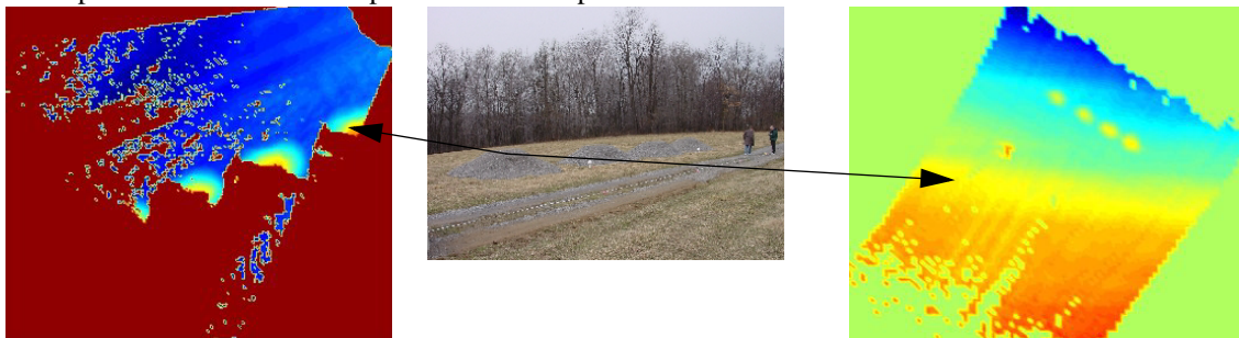
Figure 2. Data from a ground sensor (left) and a helicopter (right) shown as elevation maps. The corresponding area is shown at center.
