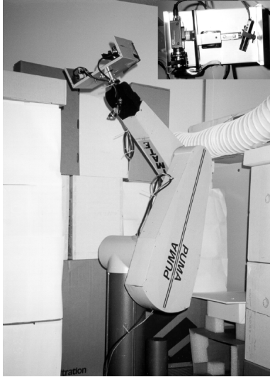
Figure 1. The experimental eye-in-hand system — a PUMA 560 with a wrist mounted area-scan laser range finder. Inset shows an enlarged view of the sensor with the camera on the left and the laser striper on the right.
