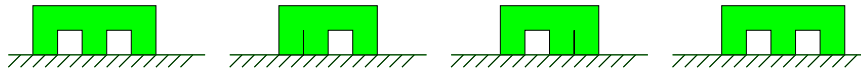
Figure 1. This figure demonstrates using shape metamorphosis for locomotion. A statically stable gait is used to translate the robot from left to right.
