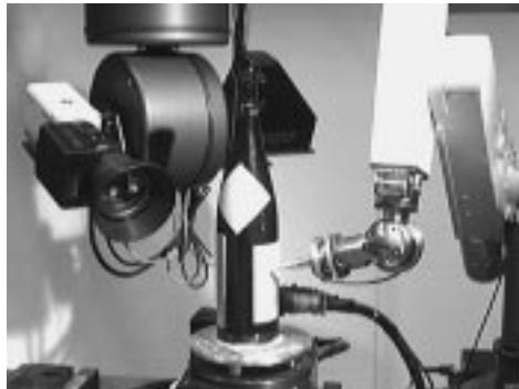
Figure 1. ACME facility being used to map surface friction and roughness of a bottle.
