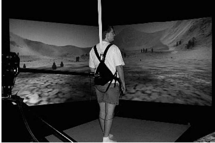
Figure 1. The Sarcos Treadport with tether attachment to a user.
