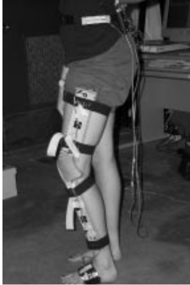
Figure 3. Marker attachment for leg joint angle measurements.
