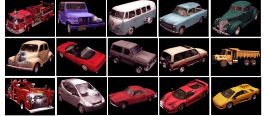
Figure 7: Examples of vehicle models used for the test. To simulate real sensor data, these facet models are converted into point clouds. Model database is constructed based on the features computed from the converted model point clouds.
